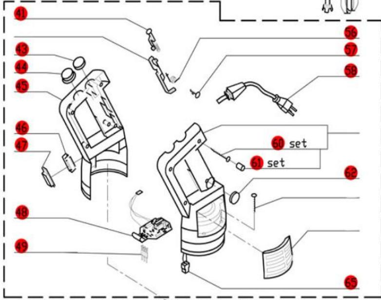
All parts within dashed lines are shipped with replacement screw caps.
